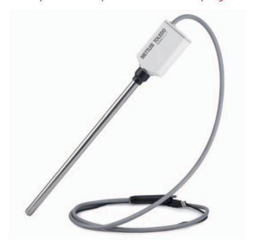
The "ParticleView V19" is a probe-based video microscope from Mettler-Toledo. This instrument visualises particles and particle mechanisms, capturing high-resolution images continuously under a wide range of process conditions without the need for sampling or offline analysis. Particles and structures often change when sampled, so visualising crystals, droplets and other particle structures inline allows transient events and elusive mechanisms that may
